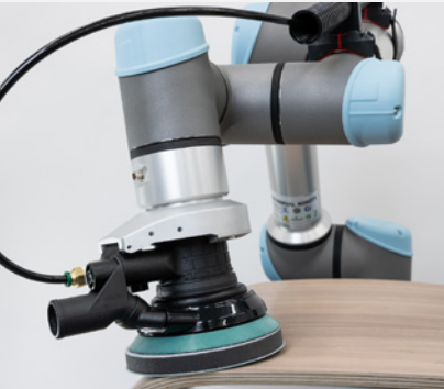
↑ Robotiq air-powered orbital sanding kit, with Finishing Copilot URCap software.
